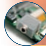
Prevention of humidity in the handset by covering the headset jack with a rubber seal
